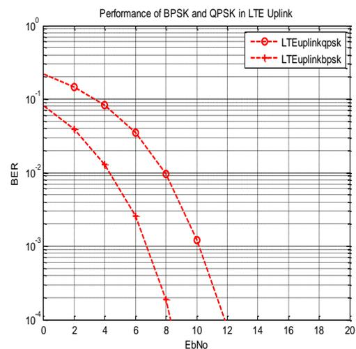
Fig.7: Performance of LTE uplink system
